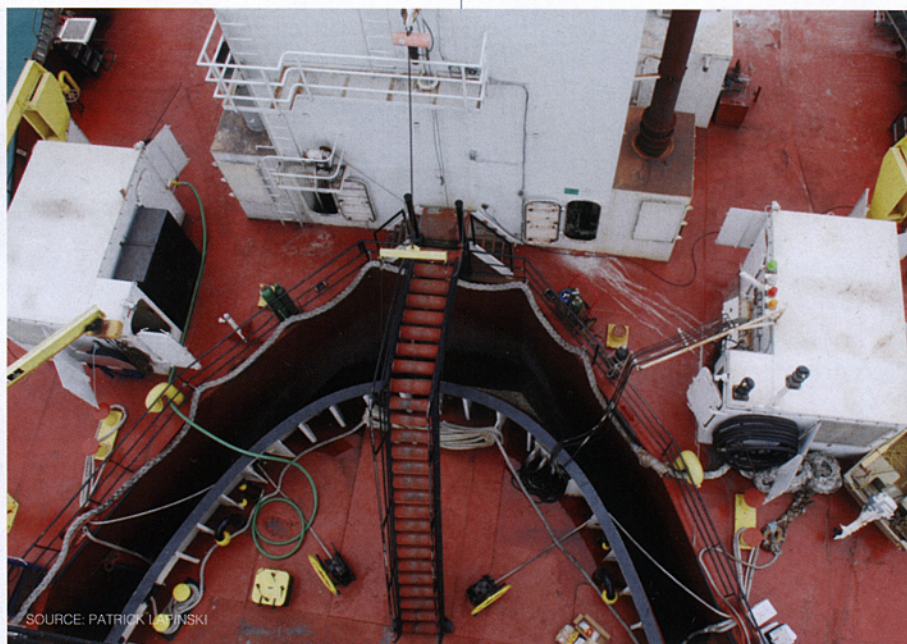
A stern notch system shown from above.
