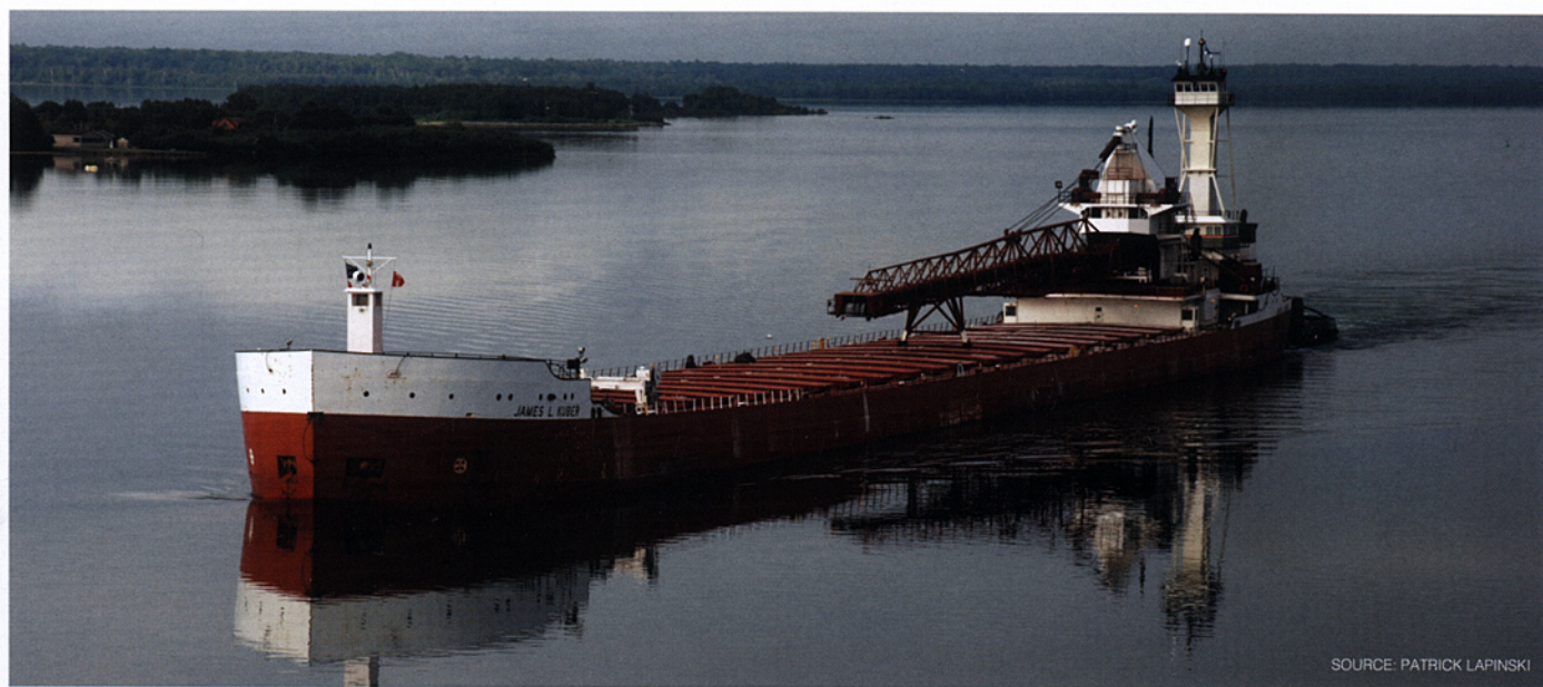
The James L. Kuber is a laker converted into an articulated tug-barge.
